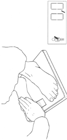
Cover the solar cells for less than one second to tare the helper's weight. Once tared, the display will show .
